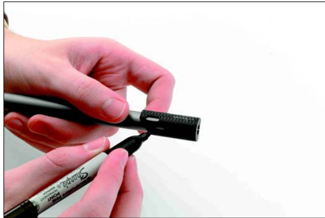
FIGURE 2A - APPLICATION OF TUBE INSPECTION MARKS USING MARKING GAGE AND PEN AS LISTED IN TABLE 2
